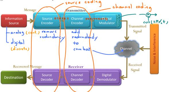
Figure 1: Basic elements of a digital communication system
